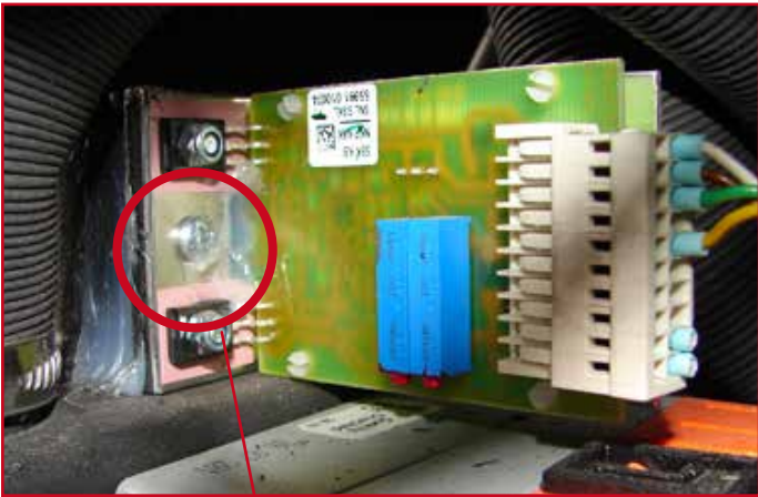
After loosening the screw the air vent sensor can be pulled out from the suction pipe.
